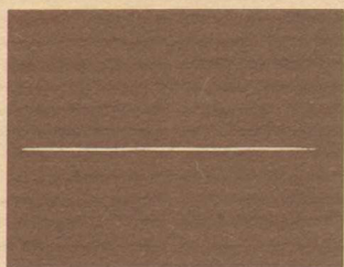
Residual Hum and Noise 102 dB below 150 Watts Scope: 5 msec/cm 10 mv/cm
