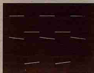
20 Hz Square Wave 150 Watts 8 Ohm Scope: 10 msec/cm Top: Input 1.0 v/cm Bottom: Output 20 v/cm
