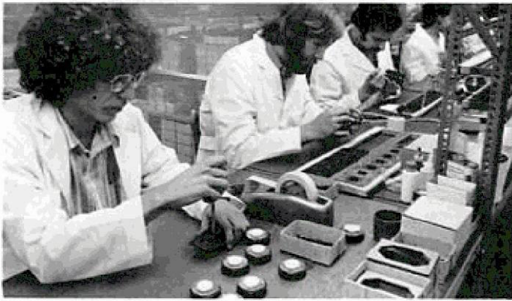
ASSEMBLY OF ADS 1" SOFTDOME TWEETERS.
