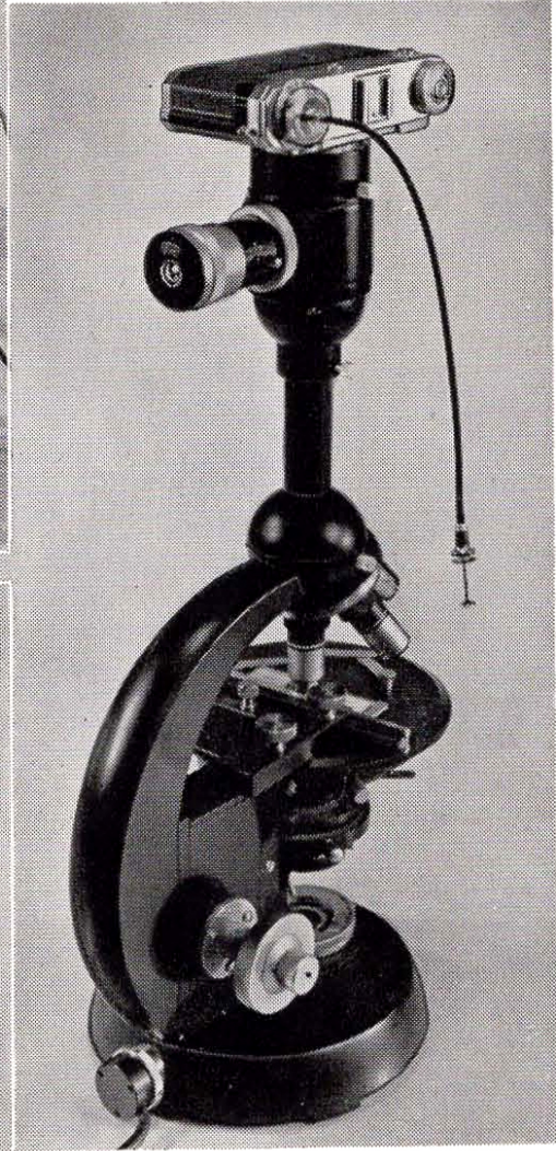
Contax mounted on microscope.
