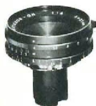
ROKKOR ULTRA - WIDE ANGLE 21mm f/4 For use with Minolta SR-7 only. Angle: 92° Minimum Focus: to 3 feet Filter mount diameter: 55mm Diaphragm: Manual pre-set
