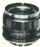
AUTO ROKKOR WIDE ANGLE 35mm f/2.8 Angle: 64° Minimum focus: to 1.25 feet Filter mount diameter: 55mm Diaphragm: Auto pre-set
