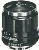
AUTO ROKKOR MEDIUM TELEPHOTO 100mm f/3.5 Angle: 24° Minimum focus: to 4 feet Filter mount diameter: 55mm Diaphragm: Auto pre-set
