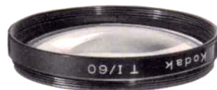
Kodak Retina 80mm Auxiliary Lens, in screw-in mount, attaches to front of Longar Lens Component, extending nearest focus point of Longar from 6½ feet down to 3½ feet for added versatility
