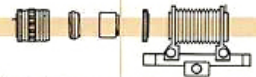
STANDARD LENS REVERSED W/ MACROPHOTO COUPLER, EXTENSION TUBE, MOUNT CONVERTER A AND BELLOWS FL
