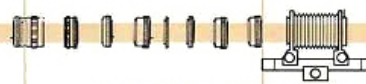
STANDARD LENS REVERSED W/ MACROPHOTO COUPLER FL, FL & M SERIES EXTENSION TUBES AND BELLOWS FL
