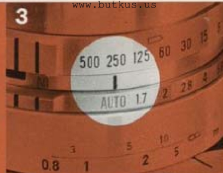
3. Set the aperture ring to AUTO mark.
