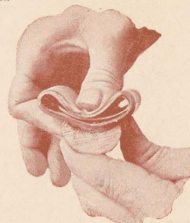
Turn the wheel so the puncture will be at the highest point. Spread the cement by pressure. Then half-inflate the tire and press the spot down to the rim again. Then inflate completely.
