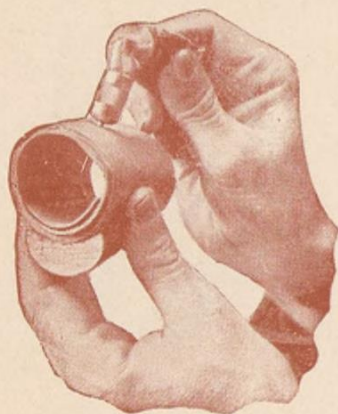
When the air has rushed out, fill the cup with cement.
