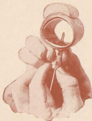
Screw in the butt end of the needle-plug, meantime turning the wheel so the cement will be forced straight up.
