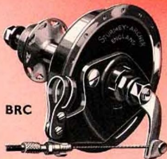
BRC REAR SINGLE SPEED HUB WITH INTERNAL EXPANDING BRAKE and cable control. Suitable for sports and sports tourist machines. BR hub similar to BRC but having rod control and suitable for tourist and roadster machines.
