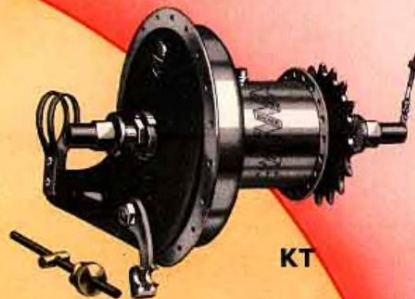
KT TANDEM STANDARD WIDE RATIO 3-SPEED HUB. Fitted with internal expanding brake with large diameter (4 1/2) brake drum. Operated by cable-cum-rod brake control, 33% increase from normal to high and 25% decrease from normal to low. Suitable for all types of tandems.
