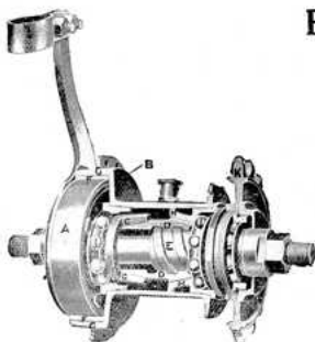
Sectional View of Eadie Coaster Brake
