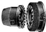
Illustration showing positive drive on Eadie Coaster Brake
